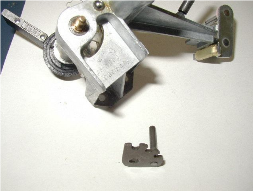
Detent plate removed...
